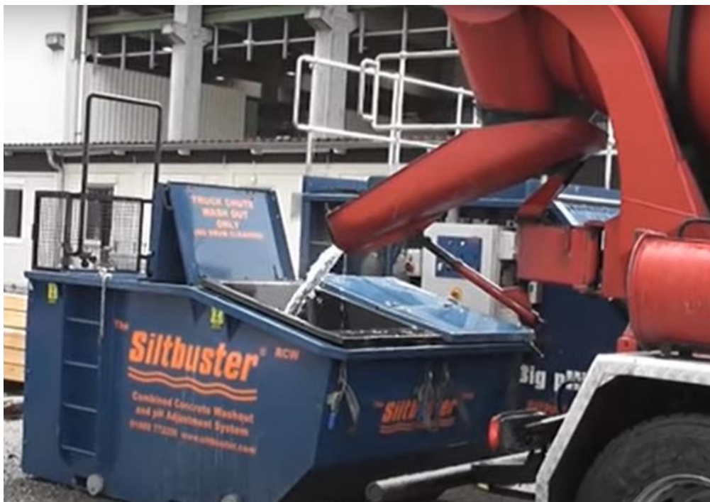
Figure 6-4 Siltbuster RCW unit in operation
